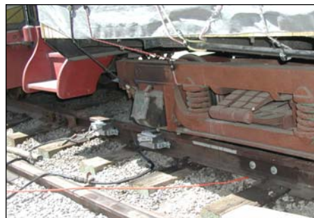
Ultrasonic probes "in action" under a passing rail car.
