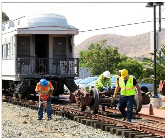
Above & below: Pullman car La Cuesta had to be shifted away from the platform to make room for loading. The tank car body came on one truck, the wheel assemblies on another. They were cleaned, lubricated, and positioned before the car body was lifted. Ted VanKlaveren, Duane Powell, Brad LaRose, and Howard Amborn worked to prepare for and carry out the move.
