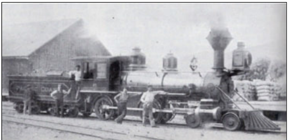
Figure 3: Engine No. 6 was a classic American 4-4-0 built by Baldwin in 1883. By 1894 it had been converted from burning wood to coal.
