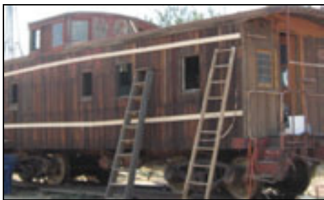
Wood strips were attached to the sides of the car to prevent pieces from falling off during transport. Photo by Dan Manion
